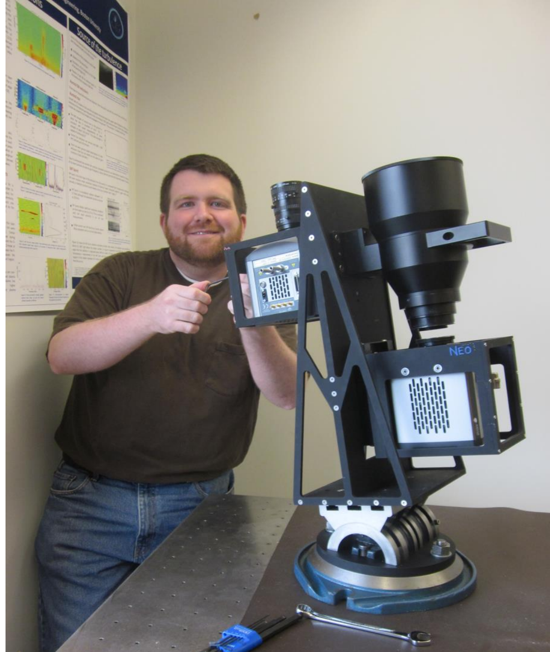
Graduate Student Michael Hirsch with the DMC camera, a sensitive high frame-rate imaging system to study the micro-scale physics governing the formation of the aurora,
