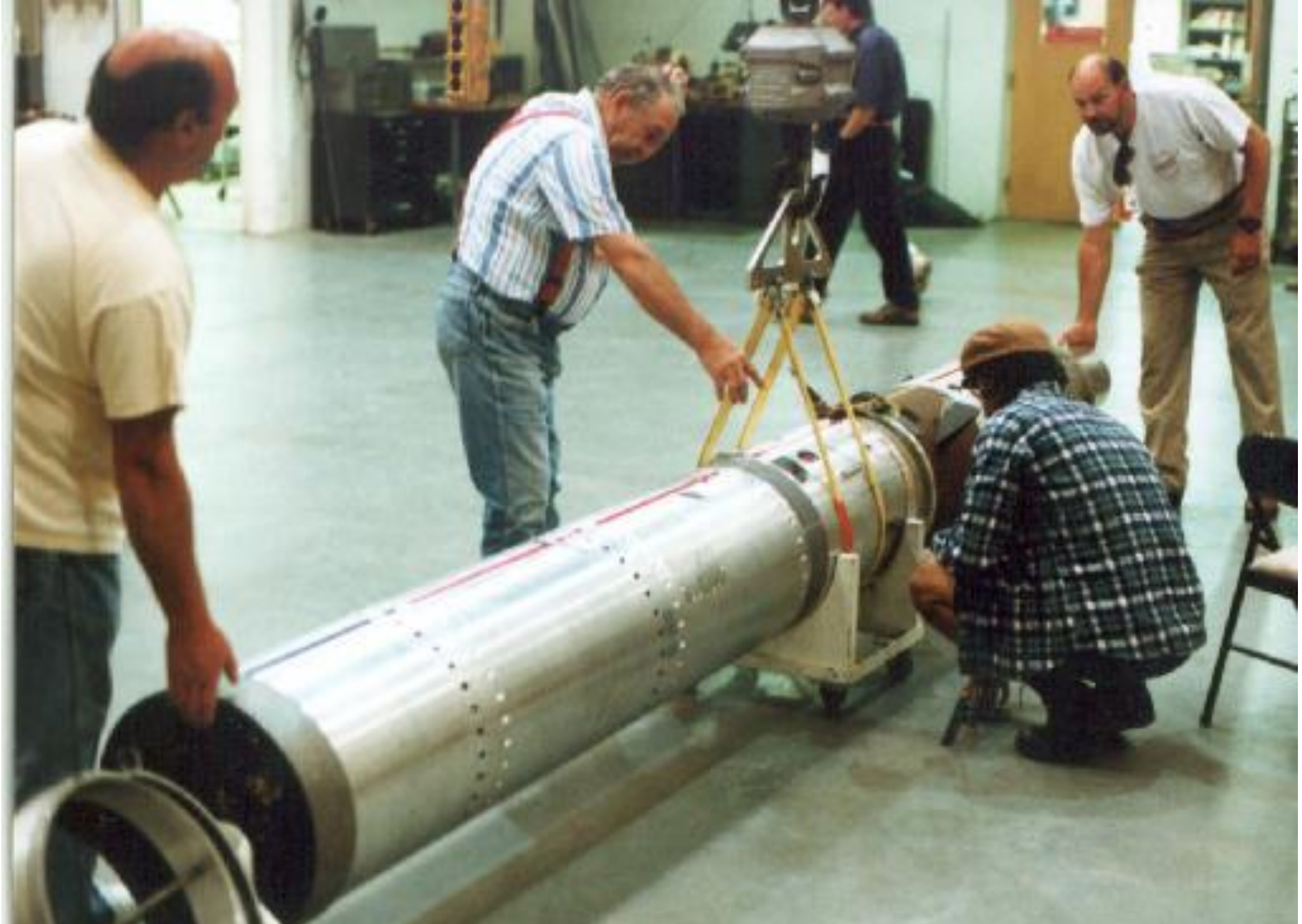
Measuring weight and center of mass of full SCARI rocket (excluding boosters)
