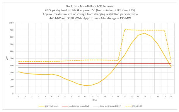
Figure 3.3-31 Tesla-Bellota LCR Sub-area 2022 Forecast Hourly Profiles
