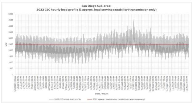
Figure 3.3-106 San Diego LCR Sub-area 2022 Load Shape and Estimated Maximum Energy Storage Capacity and Energy Based on Charging Capability Under Critical Contingency
