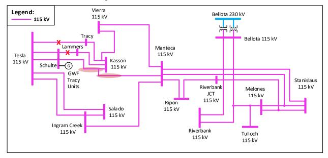
Figure 3.3-29 Tesla-Bellota LCR Sub-area
