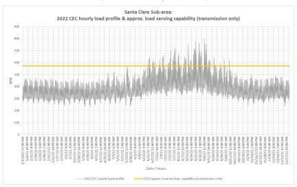
Figure 3.3-86 Santa Clara LCR Sub-area 2022 Load Shape and Estimated Maximum Energy Storage Capacity and Energy Based on Charging Capability Under Critical Contingency
