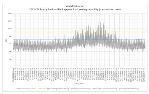
Figure 3.3-83 Vestal LCR Sub-area 2022 Load Shape and Estimated Maximum Energy Storage Capacity and Energy Based on Charging Capability Under Critical Contingency
