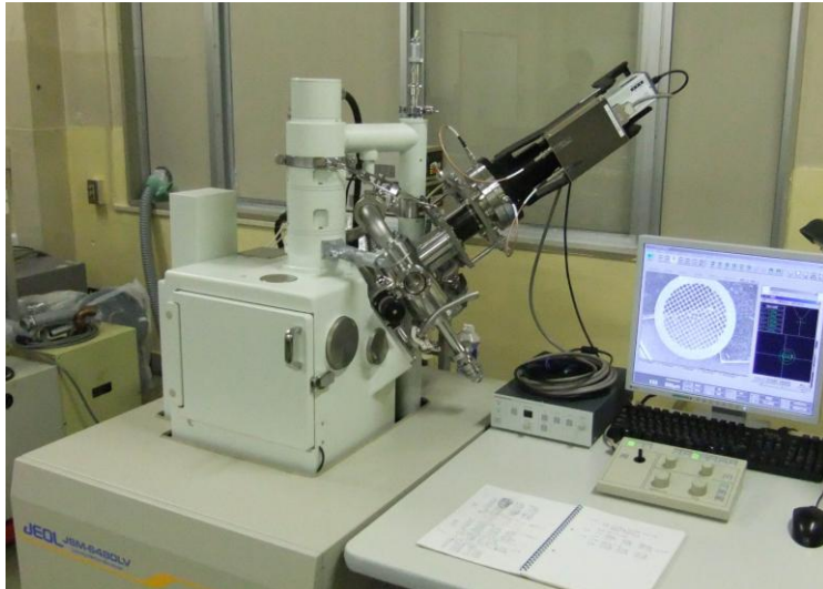
Figure 1. Photo of the newly manufactured SXES spectrometer attached to a conventional SEM (JSM-6480LV). As a detector, a multi-channel plate optically coupled with a conventional CCD camera was used.
