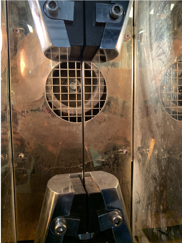
Fig. 8. Mechanical property testing under heating.
