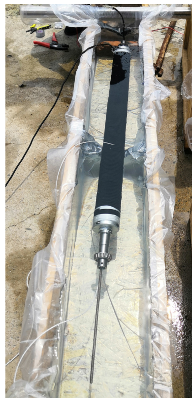
Fig. 5. Cable temperature rise testing in water under maximum operating current.
