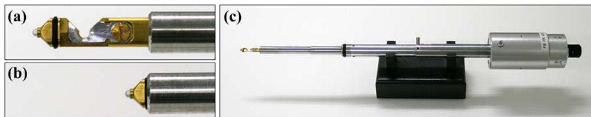
Fig. 1. The photographs of the atmosphere isolation type compatible FIB/STEM holder. (a) FIB and STEM position of the holder tip. (b) Atmosphere isolating position during the transportation of the sample between FIB and STEM. (c) The appearance of the holder.
