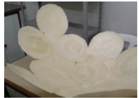
Figure 4. Gradual formation of a hemisphere by building up polymer plates 40 centimetres in diameter. Credit: Aquino, H. A.
