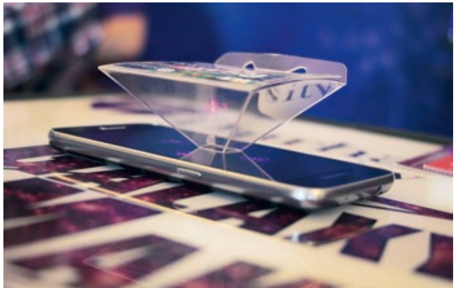
Figure 3. One of the hologram pyramids in use with a smartphone. Note the floating simulation. Credit: Josh Borrow
