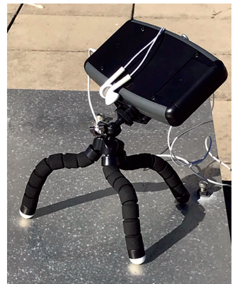
Figure 1. LightSound device on a portable tripod with headphones attached. Credit: Allyson Bieryla
