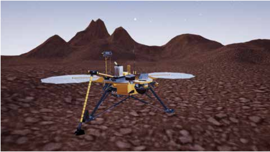
Figure 4. A 3D model of the NASA Phoenix lander that reached Mars in 2008 and conducted experiments on the presence of water and the potential habitability of Mars. Credit: Impey/Danehy/University of Arizona
