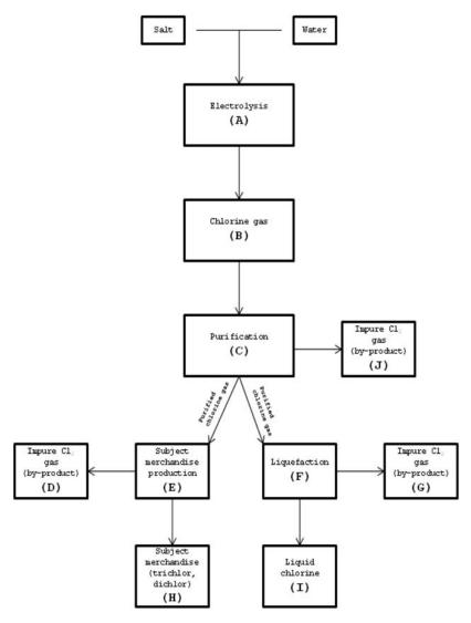
As can be seen, chlorine gas is produced by electrolysis early in the process (A, B). Thereafter, the chlorine gas is purified (C), but then the process branches into two parts. One branch results in subject merchandise (H), and impure chlorine gas (D) is discharged. No party disputes that plaintiff should receive an offset for the impure chlorine gas discharged at (D).
