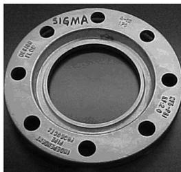
The bolt rings are described as being used specifically on HDPE (high density poly ethylene) pipes in conjunction with HDPE flange adaptors. The flange adaptors are fused by heat to the ends of the pipe. The flange adaptors provide a tighter seal but do not make a connection between the pipes. The bolt rings slip behind each of the fused flange adaptors. The rings are bolted together and serve as a clamping device to provide a tighter seal and connect the pipes together.
