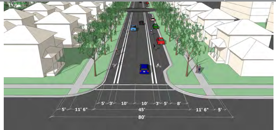
Collector - Buffered Bike Lane
