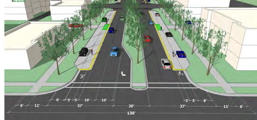
Arterial - Raised Bike Lanes with Parking
