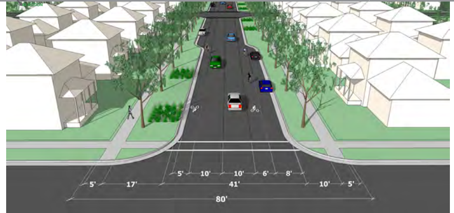
Collector - Chicane Parking
