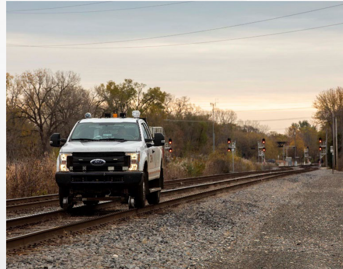
CN Hi-rail in the field: Used to patrol and inspect track
