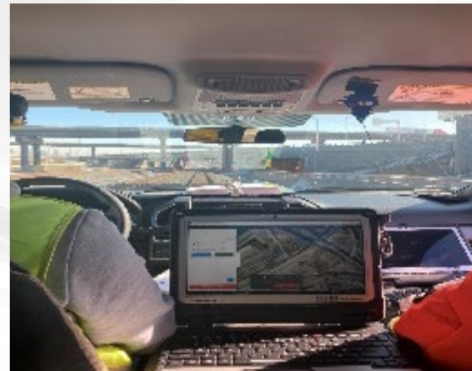
CN Hi-rail, interior: ETAV alerts Engineering employees when they approach, or exceed, their work limits
