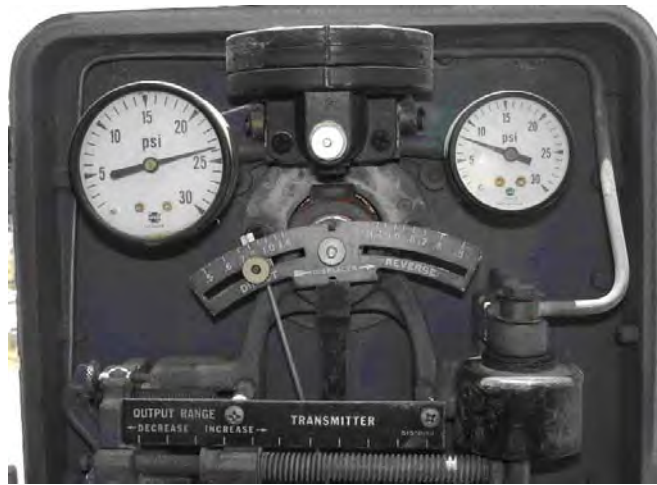
Figure S- 3. LT-5100 cabinet showing calibration set for 0.8 specific gravity
