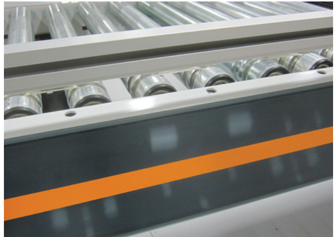
Guard rail with optional side cover
