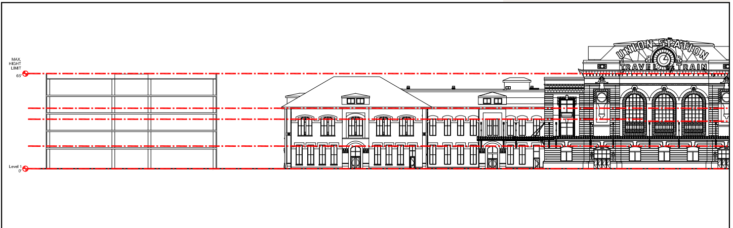
Fig 2.5: The horizontal datums and overall articulation of the facades of the historic Station building should be considered.
