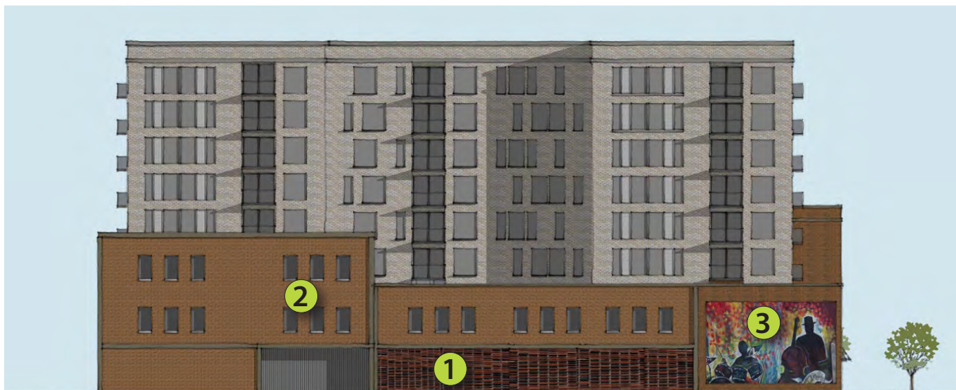
Structured parking on the alley facade of infill construction facing toward the neighborhood. Vegetative screening (1) has been limited to the ground floor with more traditional solid-to-void screening (2) above. A public art mural (3) is used on the facade that conceals the parking ramps.
