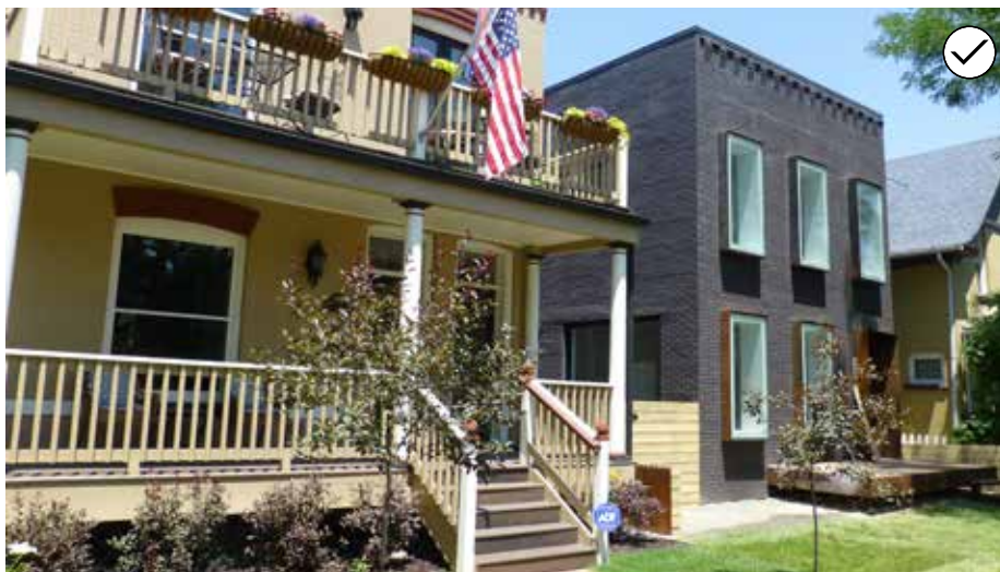
85. Design the façade to reflect typical historic proportions of height to width in the surrounding context/block.
