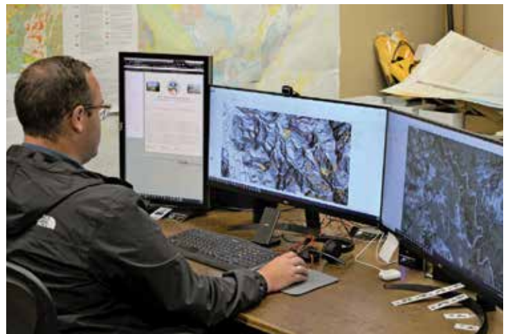
FIGURE 2. NDGS geologist Chris Maike conducting comparative analysis of landslides using two different LiDAR surface models in the GIS desktop mapping environment.
