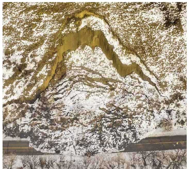
FIGURE 5. Landslide encroaching onto River Road north of Pioneer Park in Bismarck causing a week-long road closure in late December of 2019. Remedial efforts were estimated to cost about one million dollars. Geologist Levi Moxness can be seen in the lower right foreground piloting the NDGS drone used to capture this image.
