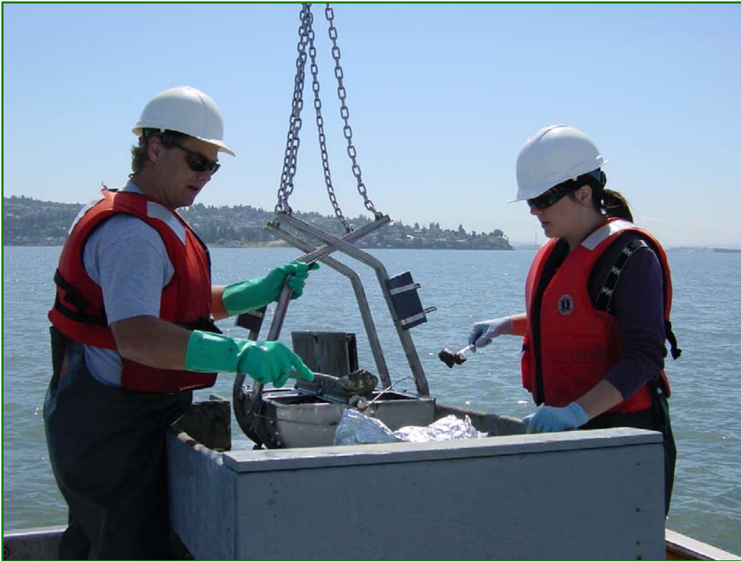
Figure 4. Stainless 0.2 m 2 dual van Veen grab sampler (left) and stainless 0.06 m 2 Gray O'Hara box core sampler (right).
