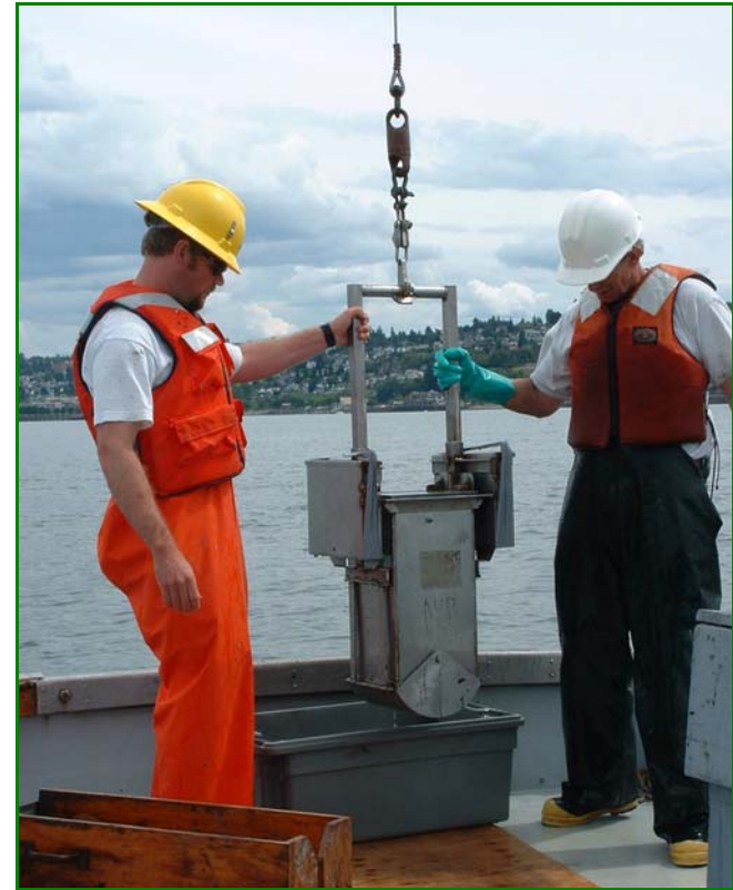
Figure 4. Stainless 0.2 m 2 dual van Veen grab sampler (left) and stainless 0.06 m 2 Gray O'Hara box core sampler (right).
