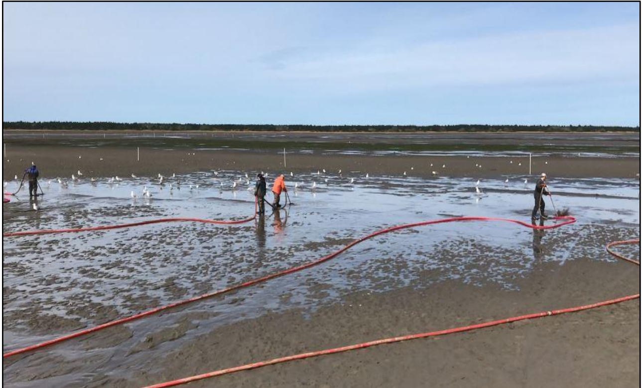
Figure 7. Liquefying an entire flooding treated plot
