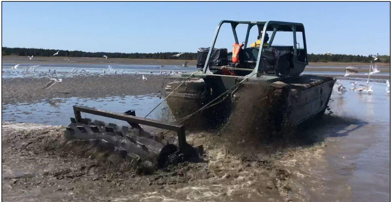
Figure 6. WADNR Marshmaster-2XL towing a roller-chopper, the implement used for “Dry Harrowing”
