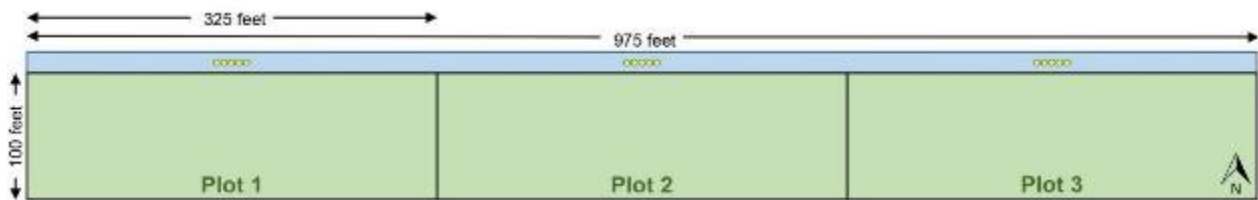
215 Figure 2. Experimental plot dimensions and layout for this study. Yellow circles represent hemispherical 216 photo point locations (five per plot). This figure represents an east-west stream orientation with the 217 treatment bank assigned to the south. 218 219 220
