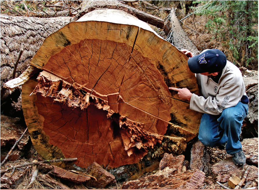
Figure 57 above. Thick sapwood is a characteristic of ponderosa pine. Young trees, which consist of nearly all sapwood, have little commercial value.
