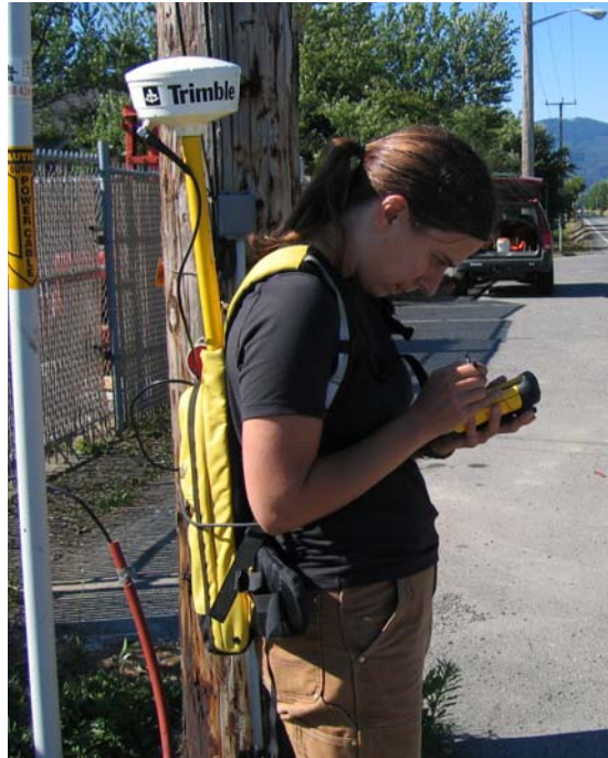
Figure 2.3. A member of the field crew using the Trimble Pro XR to collect GPS data at a survey monument
