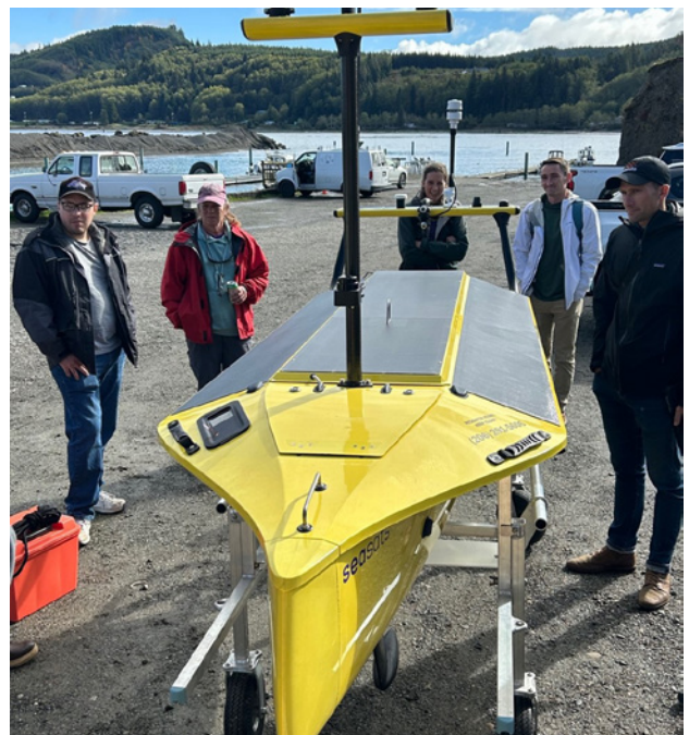
Photo 4. The Lightfish is a surface autonomous vehicle that will sample seawater at HAB “hotspots” off the coasts of Washington and Oregon to help provide an early warning of HABs making their way to coastal beaches, where they can poison shellfish and prevent harvest of clams and crabs.
