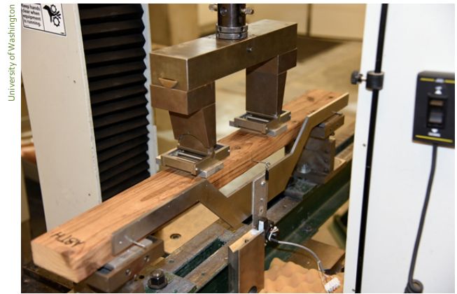
Thermally modified hemlock board mounted in the testing apparatus for the bend strength test
