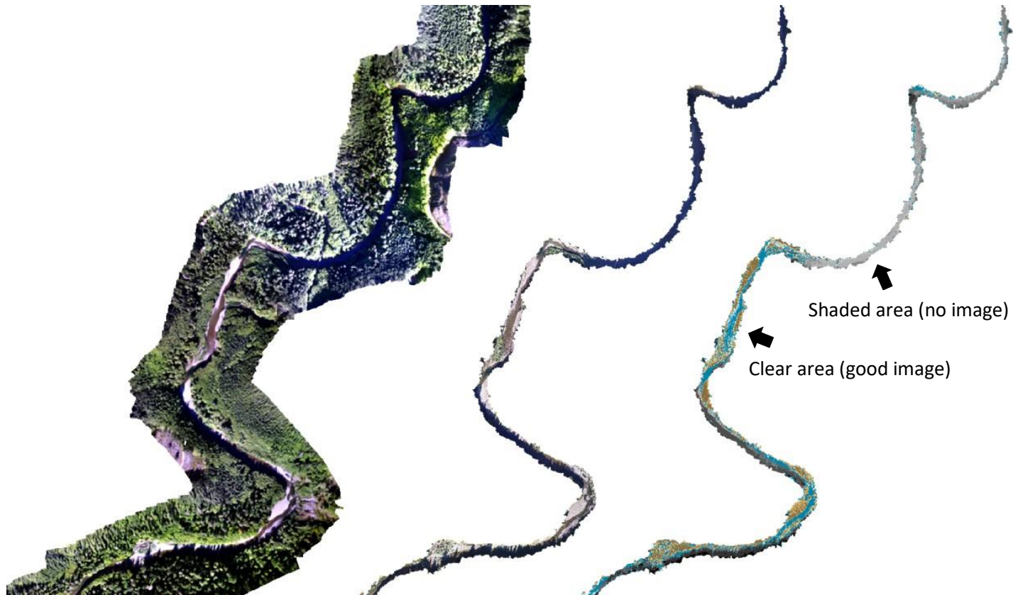
Figure 14. Processed Images taken from UAV flight over a three km section of the Clearwater River a week after snorkel and habitat survey. The image on the left is unprocessed. The middle image was clipped to include only the bankful area of a stream. The image on the right has been digitally converted after processing through ESRI's Arc Map. In the digital image greys and black represents shaded images, while blues are water and brown colors represent substrate.
