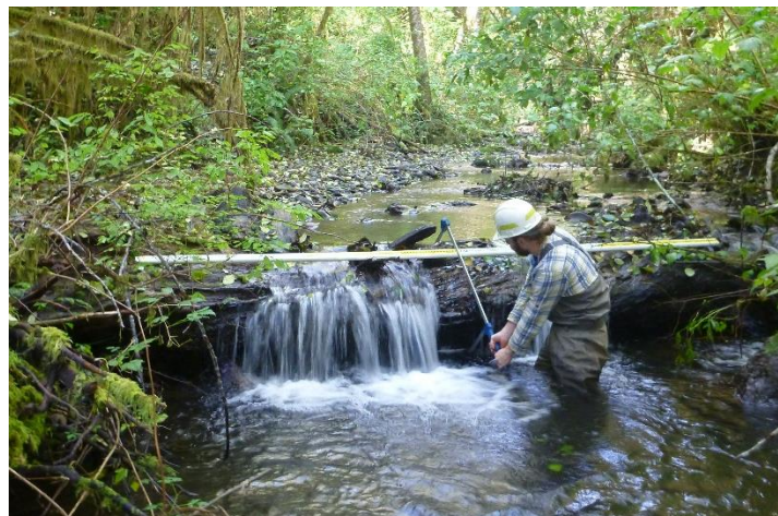
Figure 13: Measurement of In-Stream Wood. A DNR field technician uses a calipers to measure large woody debris in a stream in the OESF. Photo courtesy of Teodora Minkova.
