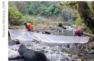
Installation of a block net along a stream in one of the experimental basins in the T3 Watershed Experiment
