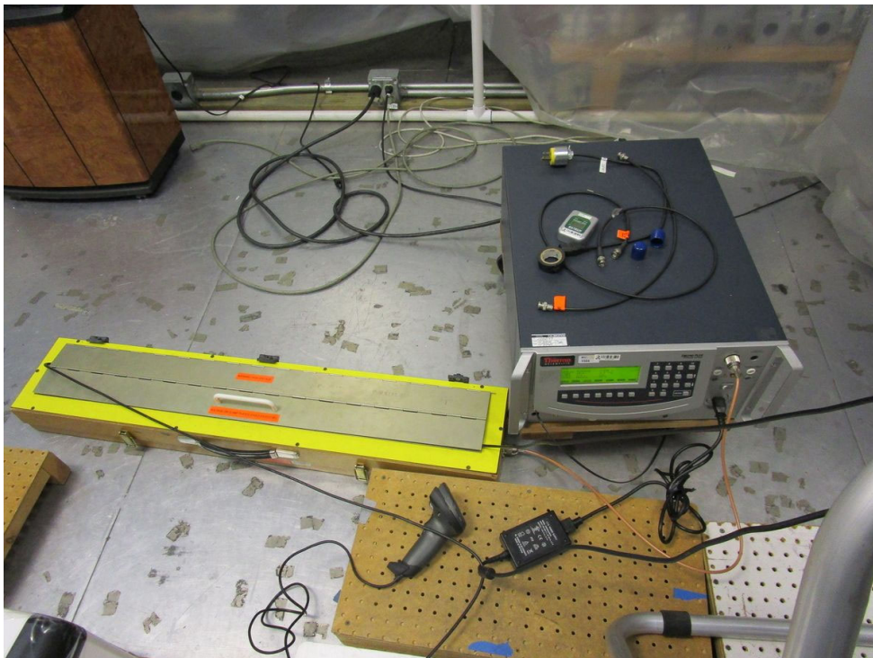
Electrical Fast Transient/Burst Setup IO_B1903101010
