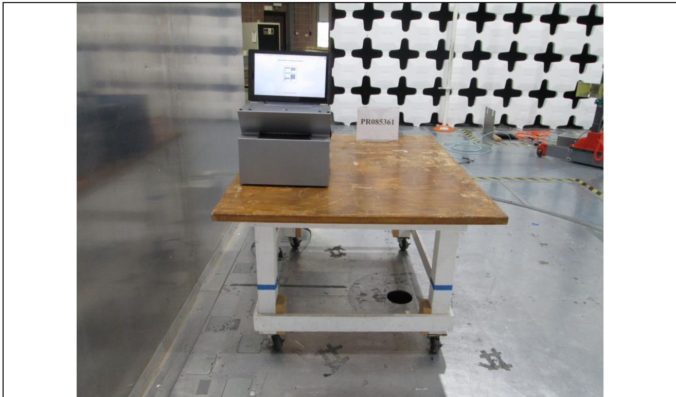
Figure B6: Conducted Emissions Test Setup – Left Side
