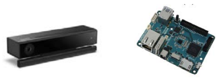
Placement of a Kinect at a ceiling, Kinect for Xbox One, Embedded computer Odroid-XU4
