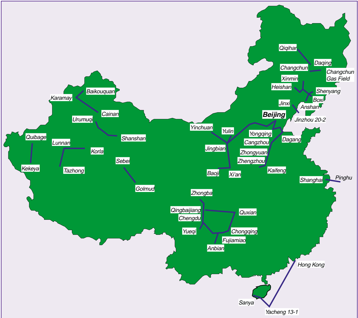
Figure 47. China's Major Natural Gas Pipelines
