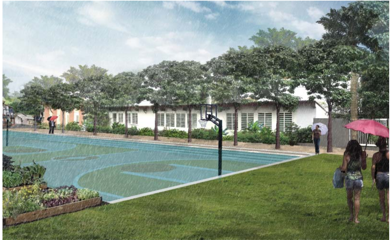
FIGURE 29 A view of the Water Plaza during a storm event. The Water Plaza can store rainwater and alleviate pressure on the gray infrastructure system.
