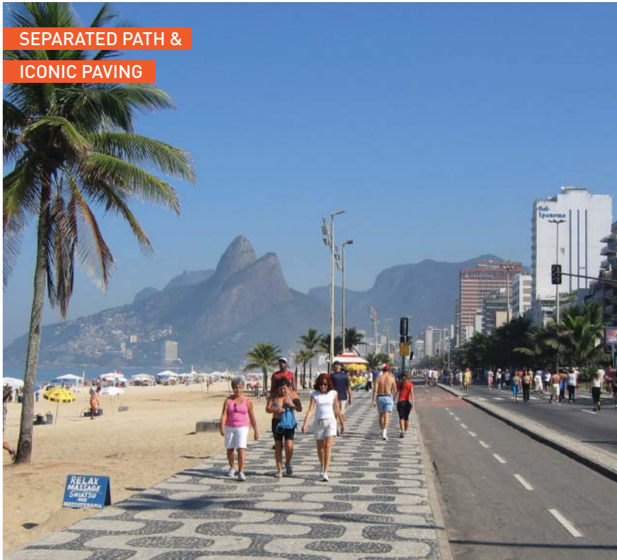
FIGURE 44 Ipanema Beach, Rio De Janeiro. The use of iconic paving pattern creates an unique sense of place and helps differentiate between pedestrian right of way and bike lanes or vehicular travel lanes.
