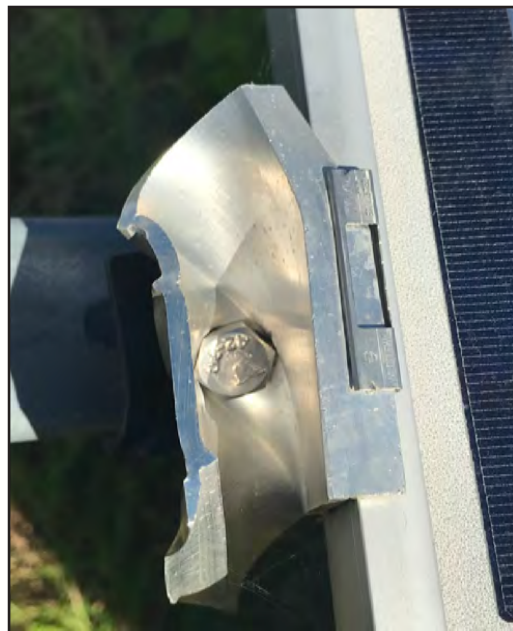
Figure 6-5: Reden solar array in Humacao: A deformed hat-shaped clip still bolted to its supporting lateral rail. The PV panel to the left was lifted out of position when the hat-shaped clip could not resist the wind uplift pressures and was bent upward.
