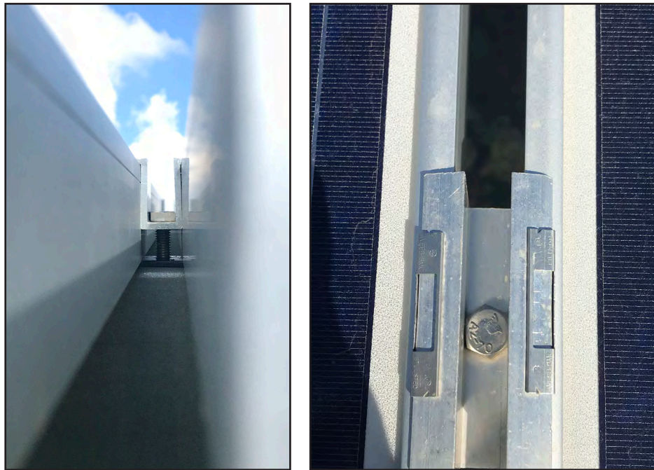
Figure 6-5: Reden solar array in Humacao: A deformed hat-shaped clip still bolted to its supporting lateral rail. The PV panel to the left was lifted out of position when the hat-shaped clip could not resist the wind uplift pressures and was bent upward.
