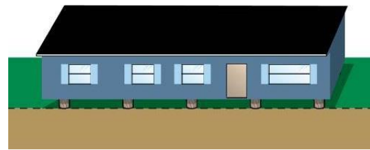
Piers and Posts
