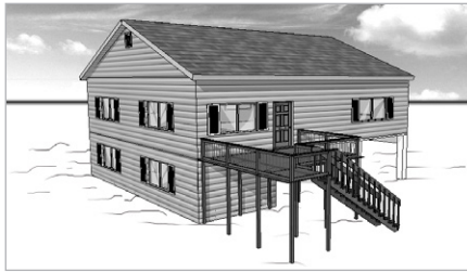
Elevated with a bedroom below the elevated floor
