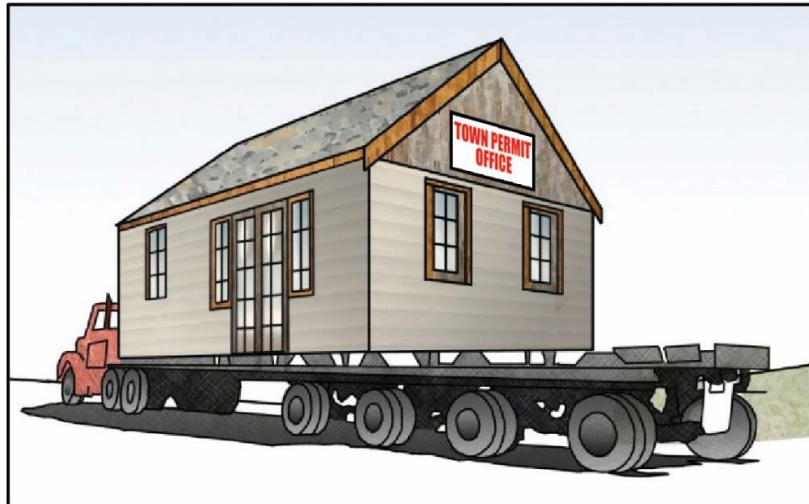
Figure 3.1.2. Relocation of a small flood-prone public building.
