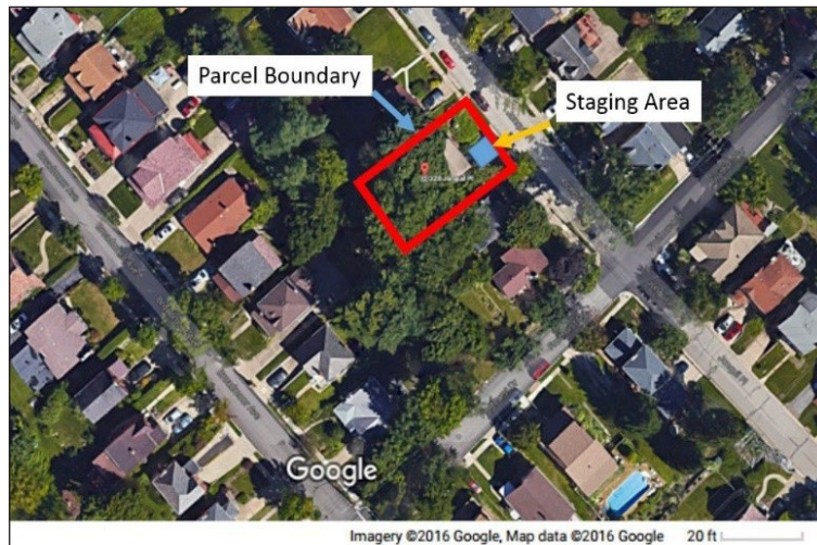
Figure 3. Example of a project site map. Map clearly shows the parcel with the structure to be retrofit, the project area, the staging area and a scale.
