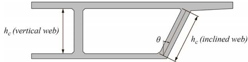
Figure 9.10 – Web Height for Equation 9.3
