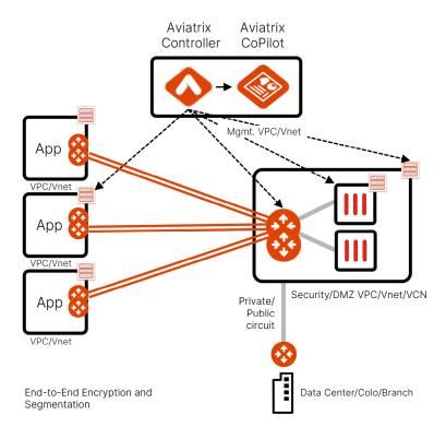
Figure 1. Aviatrix Controller manages the health and life cycle of FortiGate-VMs
