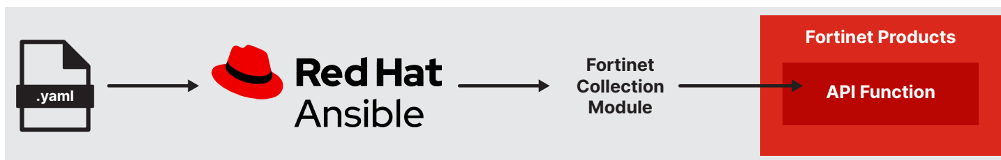
Figure 1: A YAML human-friendly configuration file, or playbook, creates an automation request to Red Hat Ansible, which uses a Fortinet module to affect change via an API call.
