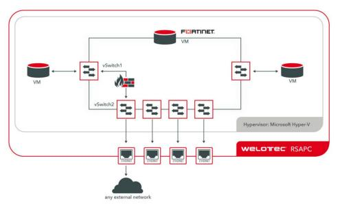
Figure 1: FortiGate VM running as virtual machine on Welotec Rugged Substation Computer beside other VMs.
