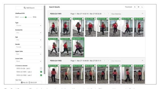
The FortiCamera Cloud edge-based analytics with smart attribute filters enables you to find a person quickly based on the color of clothing, gender, and time frame. With the Person ReID deep-learning technology, you can find the same person easily across all cameras.
