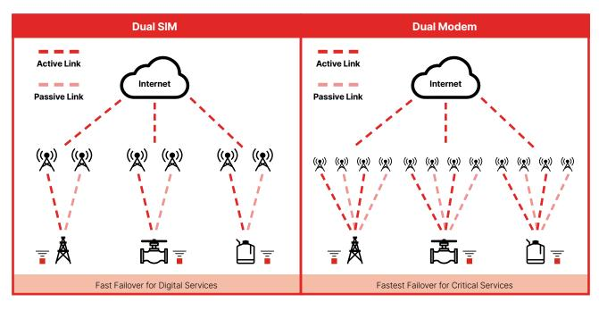
**Out-of-band management (OBM):** FortiExtender cellular gateways provide critical business continuity capabilities through the FortiExtender Cloud dashboard. FortiExtender OBM allows enterprises to continue site device management outside of the traditional provider network and deliver consistent connectivity even in the event of a wired link disaster or outage.
