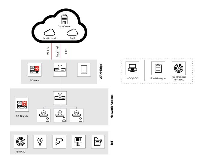
Figure 1: SD-WAN lays the foundation for organizations to extend WAN-edge transformation to SD-Branch, which consolidates networking and security into one solution.
