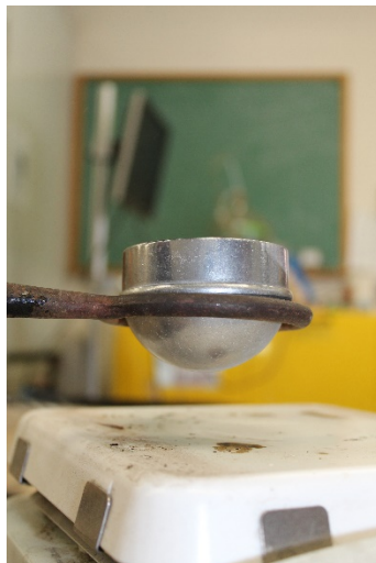
Results of water-drop demonstration. No water is visible on the electrically-heated post cap; water droplets have condensed on the combustion-heated post cap.
