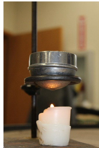
Results of water-drop demonstration. No water is visible on the electrically-heated post cap; water droplets have condensed on the combustion-heated post cap.
