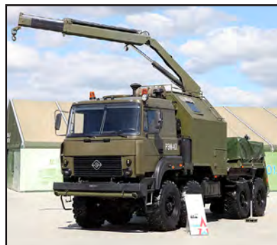
REM-KL РЭМ-КЛ Wheeled Maintenance-Recovery Vehicle
