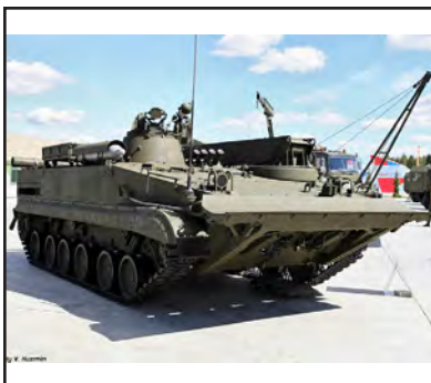
BREM-L БРЭМ-Л Armored Maintenance-Recovery Vehicle
