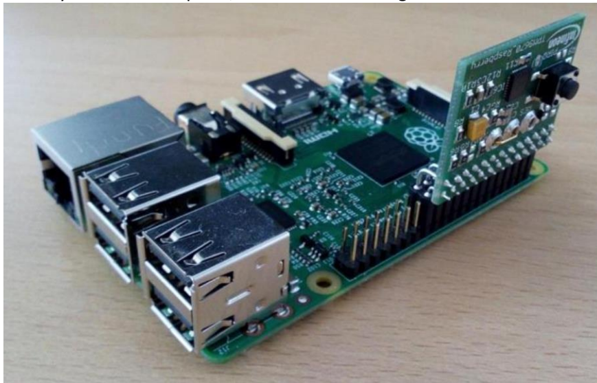
Figure 8. Iridium board installed on Raspberry Pi 3
