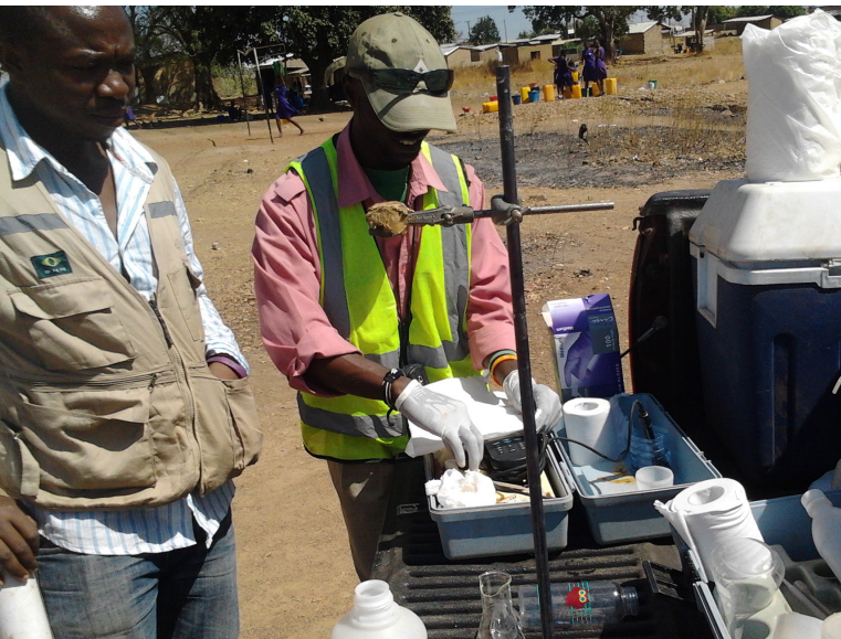
Sample preparation for tritium analysis of groundwater, Isotope Hydrology Laboratory, Ghana Atomic Energy Commission. (Photo: D. Calma/IAEA)
